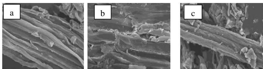
**Fig. 3 SEM images of (a) Ground Teak wood powder, (b) Bleached teakwood dry pulp and (c) Dry Cellulose Nano Fibrils.**
