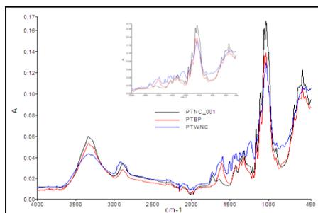
**Fig. 1 FTIR spectra of ground Teak wood powder, bleached teakwood dry pulp and dry Cellulose Nano Fibrils in the region of 4000-450cm<sup>-1</sup>. Inset spectra in the region of 1800 – 450 cm<sup>-1</sup>.**
