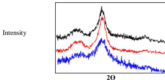
**Fig. 2 XRD Pattern of ground Teak wood powder, bleached teakwood dry pulp and dry Cellulose Nano Fibrils.**
