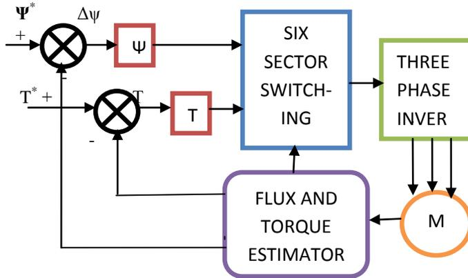
Figure 2 shows block diagram of DTC switching table concept
