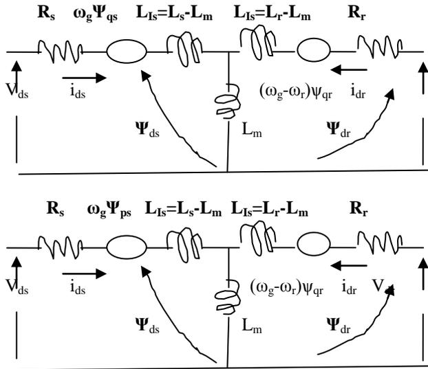
Figure.1 Dynamic d-q equivalent circuits of an asynchronous drive (a) d-axis, (b) q-axis
