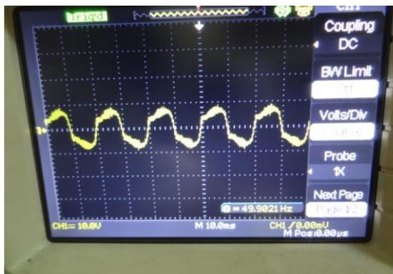
Fig.17. Experimental Waveform for Generator side voltage, CH2=10V/div
