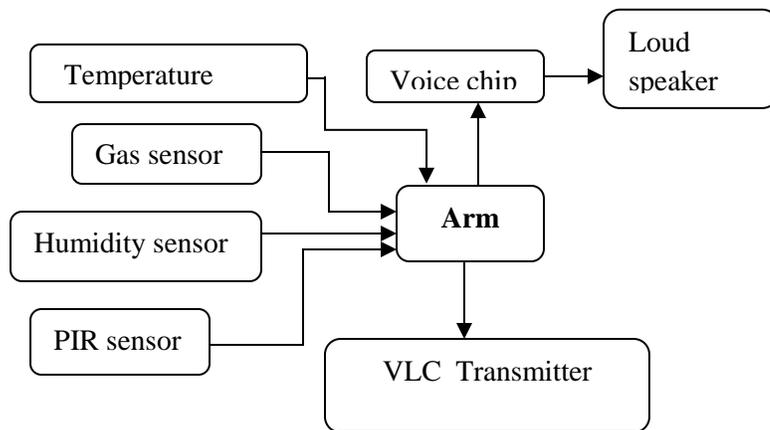
*Fig 7.1.1.1 Proposed Block Diagram for Mine Section*
