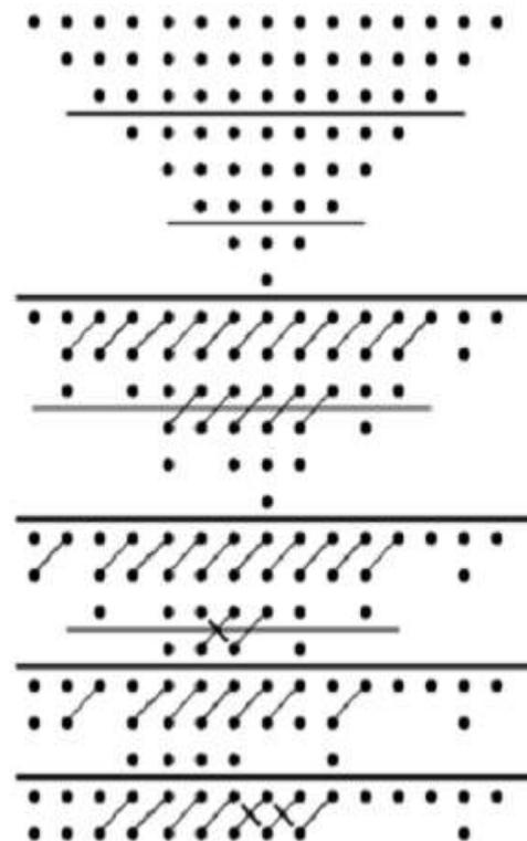
Fig.4. Proposed Design for modified Wallace multiplier 8x8
