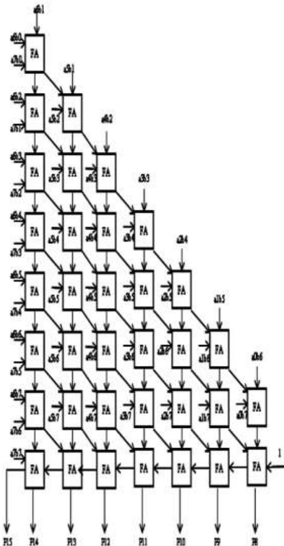
Fig.3. The architecture of a truncated 8x8-bit parallel multiplier.
