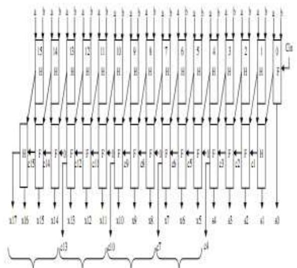
Fig.6. Modified carry save adder.
