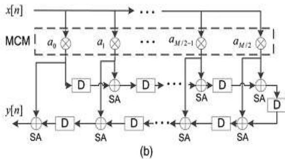
Fig.1. Structures of Linear-Phase Even-Order FIR Filters: (a) Direct Form and (b) Transposed Form.
