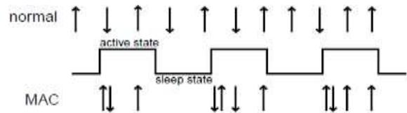
Figure 1: The MAC duty cycle; the arrows indicate transmitted and received messages; note that messages come closer together.
