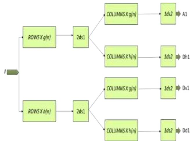
Fig.. 2. Shows 2-D-DWT decomposition, here 2ds1 indicates that rows are down sampled by two and columns by one. 1ds2 indicates that rows are down sampled by one and columns by two. The “x” operator indicates convolution operation.
