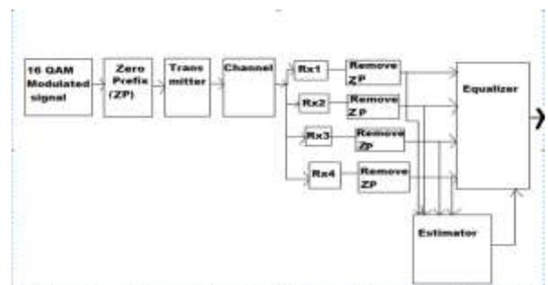
Fig.2 System Block Diagram for Simulation.
