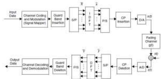
Fig 1 A Digital Implementation of a Baseband OFDM System
