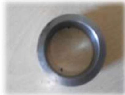
Fig 5.1. Thrust washer
