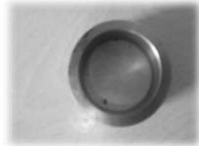
Fig 5.3.Thrust washer
