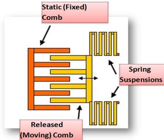
**Figure 4 Differential capacitor sensor**
