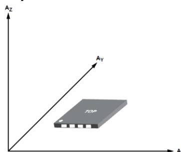
**Figure 5 Sensor Axis**
