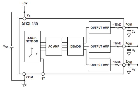
Figure 3 Block Diagram of ADXL335
