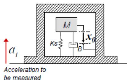
Figure 1 Accelerometer Principle
