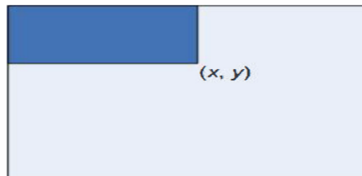
Figure 1. The shaded region represents the sum of pixels up to the position (x, y) of the image.
